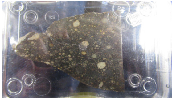
Chondrite , in general, any stony meteorite characterized by the presence of chondrules.
