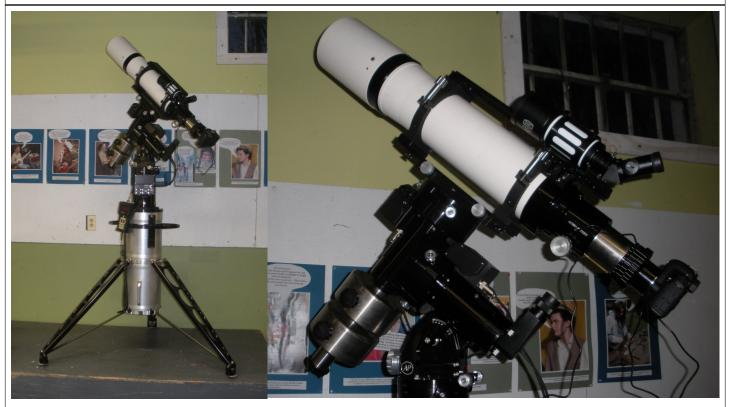
Kirk Rogers brought his new toy to the April meeting. He calls it his "Portable Astro-imaging Instrument." It incorporates old and new hardware. The old, is the tripod and the f/6 130 Astro Physics refractor. The new is the mount and CP3 Control Box that sits between the tripod and telescope (close-up shown in right image). Also new is a DSLR Canon camera which was modified. WOW!
